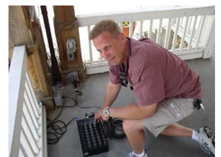
Gerry Tacker, director of operations, is shown connecting an audio input to the LightViper stage box; the unit's optical output is then plugged into a separate, weatherproofed receptacle that routes the audio over 150 feet of fiber cable to the FOH mixing position.
